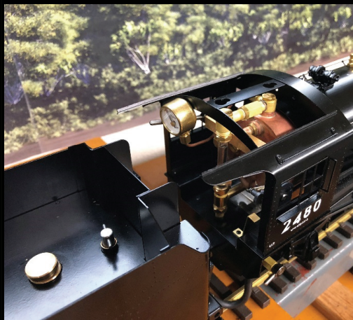
Featuring removeable cab roof and lift-off alcohol tank for easy refueling.
