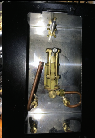
Kingston valve and larger hand pump. Easy to connect water tank car.
